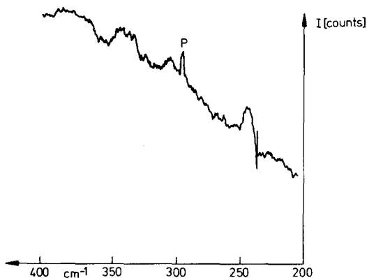
FIG. 4. Raman spectrum in the range of 200–400 \text{cm}^{-1} . P_{\text{ads}} = 100 Torr; T_{\text{ads}} = 20^\circ\text{C} . P, Laser plasma.
